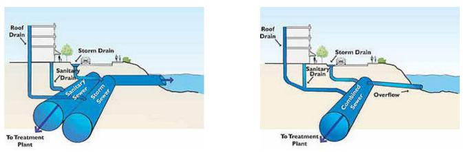
Figure 7. Schematics of (A-Above Left) Separate Sewer Systems and (B-Above Right) Combined Sewer Systems. (Source: <u>San</u> Francisco Better Streets Plan)
