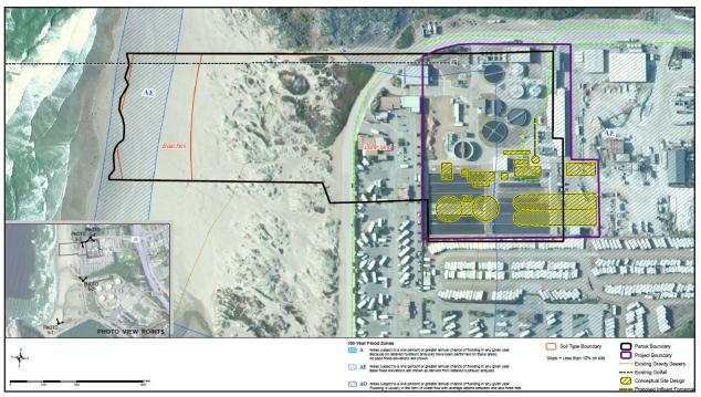
Figure E-9. Project plans for the denied Morro Bay Cayucos Wastewater Treatment Plant showing flooding hazards.
