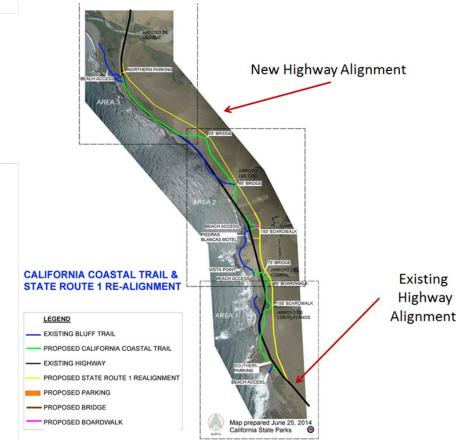
Figure E-11. Project plans showing realignment of Highway 1.
