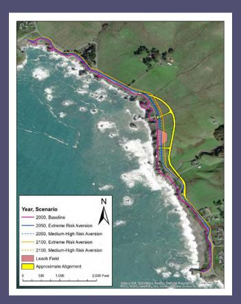
Smith River in Del Norte County. The analysis showed that even extreme storm flooding combined with the H++ scenario for sea level rise would be lower than the originally proposed bridge elevation, and no additional project changes or follow-up adaptation planning was required.
